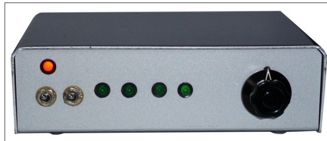
The 12 V control unit for the two Flag antenna relays is quite straightforward consisting of a power switch, a switch for choosing between two receivers and a 3 pole 4 position rotary switch. LED indicators show Power on and the actual Flag antenna direction.
