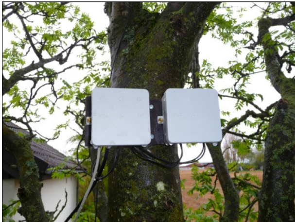
Picture showing the two plastic boxes (10x10 cm) with relay and toroid attached to a small plywood board.
