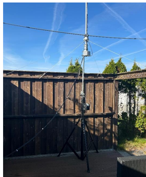
Fig.3: The "microFLAG" with rotator and thrust bearing on my small patio.
