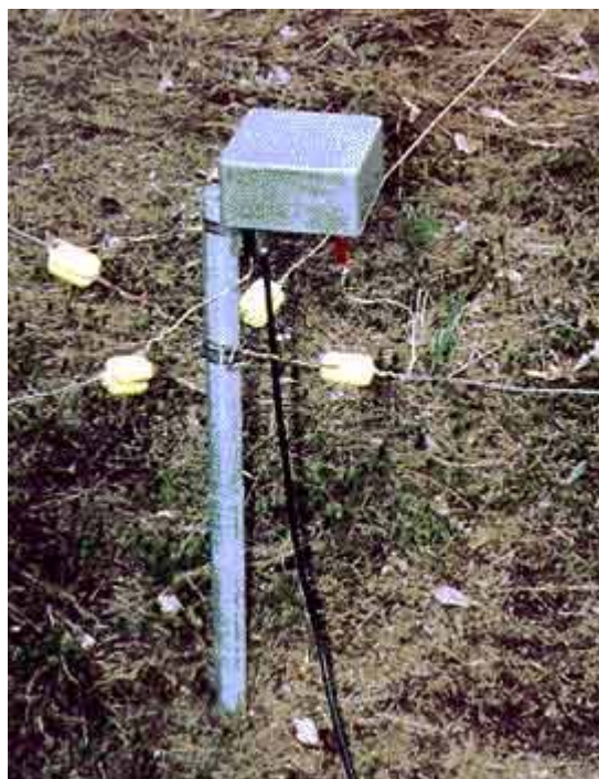
Figure 4—A photo of the central connection point at the base of a two-loop system, as installed at K9AY.
